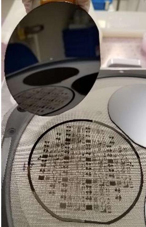
Figure 7. 100mm TGV glass wafer with conformal gold fill and front-side RDL, after debonding onto dicing tape. The clean silicon handle wafer is also shown.
