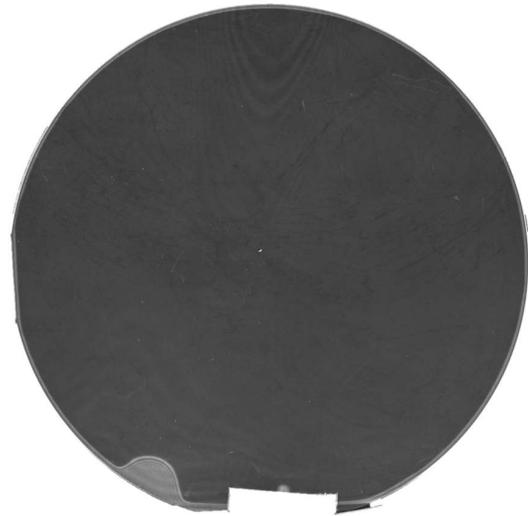
Figure 8. Fused silica after grind and polish, with the newly polished side bonded to a Si handle to visualize quality of the bond. (Collaboration with Disco Corporation.)
